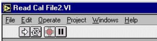
The arrow is RUN. The RED Button will stop the program. Other buttons are not to be used. Online control feature help is enabled with the HELP:Show Help checkmark. This buttons are not normally used.
