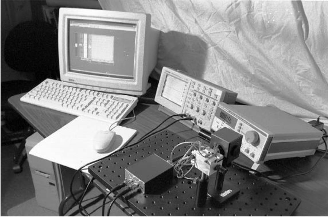
System Example: PC, Tek TDS 210 scope, ILX -LDP-3811, Custom Pre-amp, Laser mount, an Integrating sphere with detector (cube). Actual components may vary with your systems. This is a photo of the original development system. The Tek digital scope, ILX LDP-3811 CW/Pulse Laser Current Source, Voltage monitor, light pre-amp, laser mount, and integrating sphere assembly are shown. A small optical plate supports the mounts and other mechanical components.
